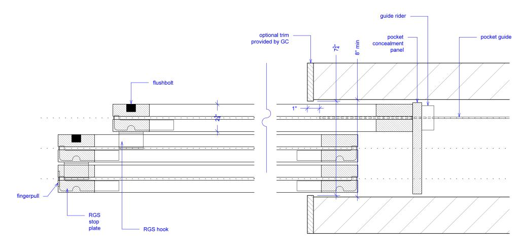
Guide rider is a block with a slit for the pocket guide; it allows for full extension, attach to bottom of concealment panel.
