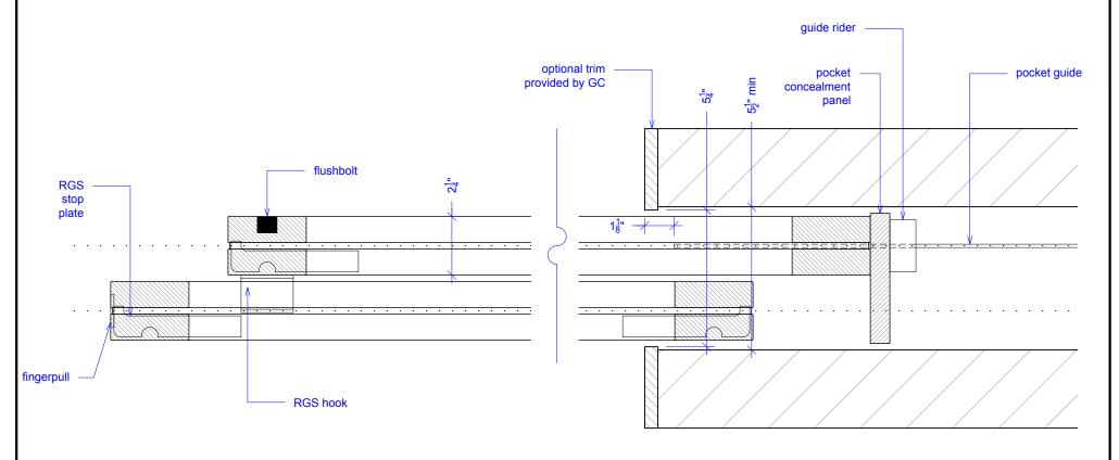
Guide rider is a block with a slit for the pocket guide; it allows for full extension, attach to bottom of concealment panel.
