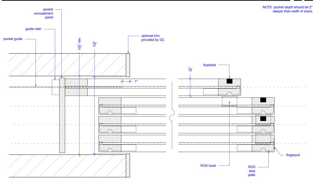
Guide rider is a block with a slit for the pocket guide; it allows for full extension, attach to bottom of concealment panel.
