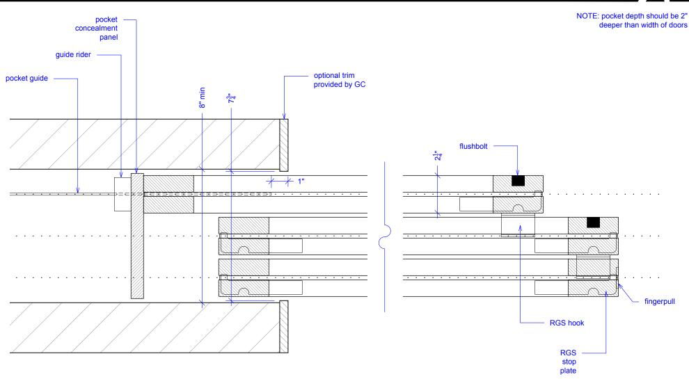
Guide rider is a block with a slit for the pocket guide; it allows for full extension, attach to bottom of concealment panel.
