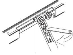
9. Insert hinges into premortised slots and attach with screws – do not over-tighten
