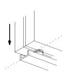
Adjust height of blind levelers with allen key
