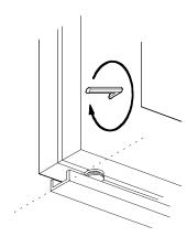
For continuous run of fixed panels be sure to use single piece of top and bottom guide to ensure alignment.
