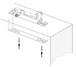
Attach ball catch receiving plate to top of door
