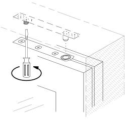
Adjust ball catch as needed by threading up or down
